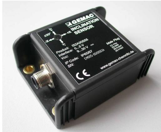
The inclination sensor IS1A xx P58 enables, depending on type, the one-channel measurement of inclinations in the ranges  $\pm 10^\circ$ ,  $\pm 45^\circ$  or  $\pm 60^\circ$ . The inclination sensor IS2A xx P58 includes two channels. The full-scale readings are calibrated factory-made at  $25^\circ\text{C}$ . The compact and robust design makes the sensor a suitable angle measurement device in rough environments for different applications in industry and automotive technology.
