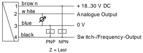
It is recommended to use shielded cable < 30 m, supply lines < 10 m
