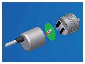
shaft rotates through a certain angle, the magnetic polarity in a 'Wiegand wire' suddenly changes, inducing a brief voltage spike in a coil surrounding the wire. This pulse both marks a rotation of the shaft and powers the electronic circuitry that records the event. The Wiegand effect occurs reliably even with very slow rotations and requires no backup batteries.
