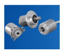
To measure rotary movements or rotary displacements, an absolute magnetic rotary encoder can be used. The contact-free measuring sensor stage of the MCD Sensor does not have any abrasion. The Sensor can be connected directly to digital control units via SSI, CANopen or Analog Interface.
