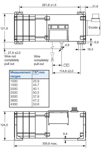
All details in mm and dependent on the encoder configuration.
